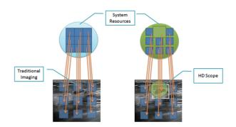
Figure 1: Traditional image (left): the imaging resources are uniformly and equally distributed through the whole field of view; HD Scope image (right): more imaging resources are assigned to the ROI
