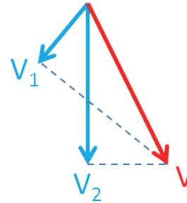
Fig. 3: Example for velocity obtained from two beams. Both the velocity and direction are obtained from an angle compounding technique, where  $V$  is the compounding velocity, and  $V_1$  and  $V_2$  are Doppler measured velocities.
