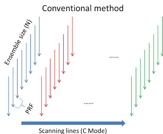
Fig. 1: Scan sequence (line-by-line) of conventional CFM
