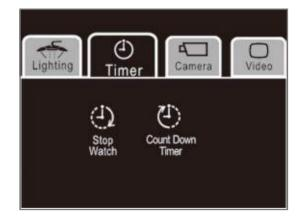
A timer function can be used to notify the surgical team of the elapsed time and a count-down alert is particularly useful for time management.
