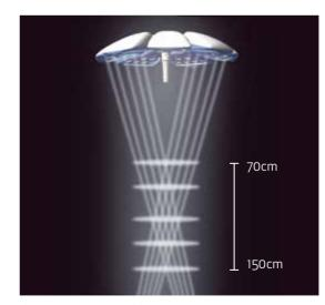
An innovative focus adjustment system can focus light from the 7 petals onto one spot to form a clear, abundant, even field of brilliance on the surgical area.
